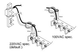
The white wire is connected to #1 and the black #2 in 220 VAC sets. Both white and black wire are connected to #1 in 115 VAC sets.
