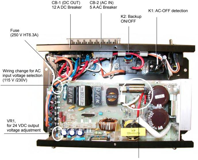
Jumper Wire for AC input voltage selection (115 V/230 V) (note)
